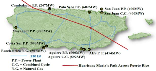
Figure 12 - Hurricane María's path across Puerto Rico and the Main transmission and generation assets of Puerto Rico's power grid (Source: Hurricane María Effects on Puerto Rico Electric Power Infrastructure- IEEE)
