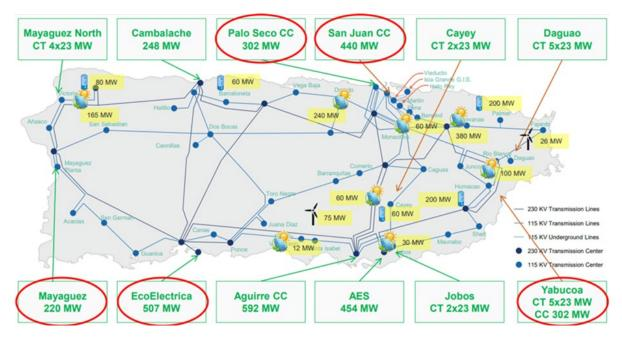
Figure 5 - Map of Puerto Rico main Electric Power Generation and Transmission Infrastructure (Source: Fiscal Plan for the Puerto Rico Electric Power Authority, as certified by the Financial Oversight and Management Board for Puerto Rico on June 27, 2019)
