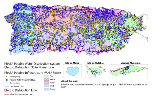
Figure 34 - PRASA Potable Water Distribution System & Electric Distribution 38KV Power Line
